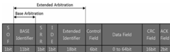
Fig.1. Data frame format of CAN 2.0B protocol.
