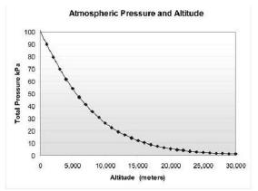
The above picture clearly indicates that, the atmospheric pressure falls down proportionate to the increase in altitude. These charts can be used in emergency to determine the altitude of aircraft.
